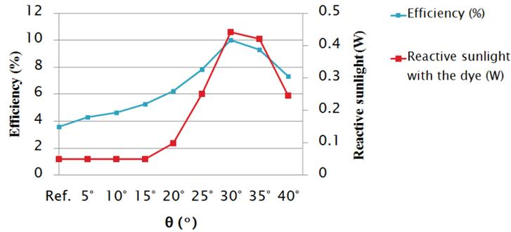
Fig. 9. Efficiency-curves of the DSSC with respect to the amount of sunlight reacting the dye.
