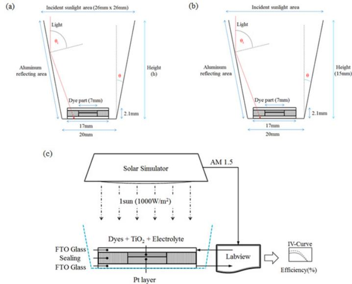
Fig. 5. (a) Experimental schematic for a fixed area of incident light. (b) Experimental schematic for varying areas of incident light. (c) Concept of test apparatus used to measure characteristics of a DSSC.
