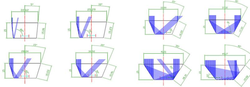
Fig. 7. Light simulations for a fixed vertical height of the reflector.
