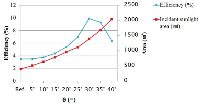
Fig. 8. Efficiency-curves of the DSSC with respect to the incident sunlight area.
