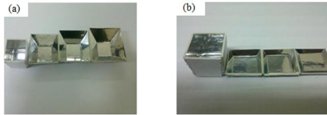
Fig. 2. (a) Manufactured reflectors with a fixed area of incident light. (b) Manufactured reflectors with various of incident light.
