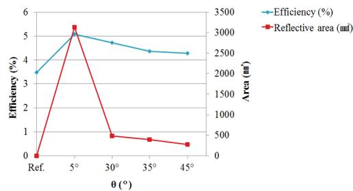
**Fig. 6. Efficiency-curves of DSSC with respect to the reflective area**
