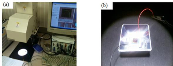
Fig. 3. (a) Test apparatus used to measure characteristics of dye-sensitized solar cell. (b) Fabricated DSSC.
