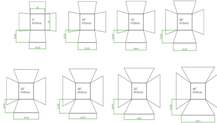
Fig. 1. Reflective condenser plate design.
